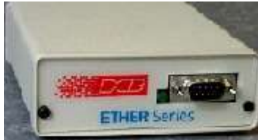
Puente entre TCP/IP, AppleTalk, DecNet, NetBeui y Ethernet Interfaces 10/100BaseT Ethernet y RS-232/422/485
