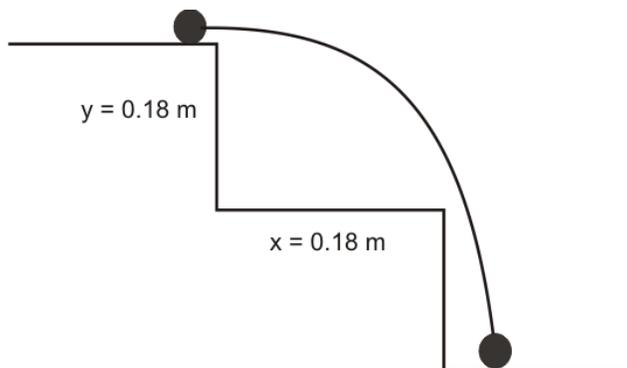
Utilizando  $y = \frac{g \cdot t^2}{2}$  tenemos:  $2(0.18\text{m}) = 9.8\text{m/s}^2 \cdot t^2 \rightarrow t = 0.189\text{s}$
