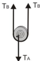
$$\sum F : 2T_B - T_A = 0 \text{ (masa polea despreciable)} \quad 4)$$
